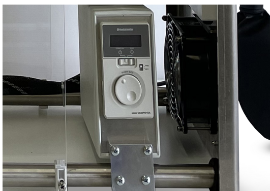
Respiratory frequency can be set on the digital regulator to reproduce resting to high respiratory rates
