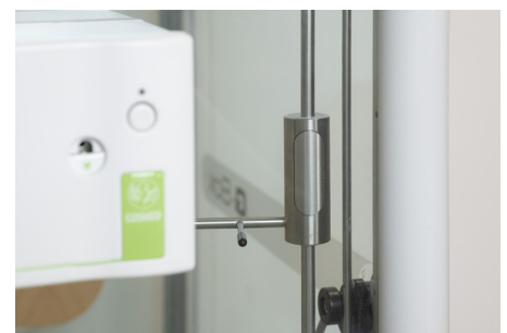
Arm with quick release mechanism for one-hand adjustment.
